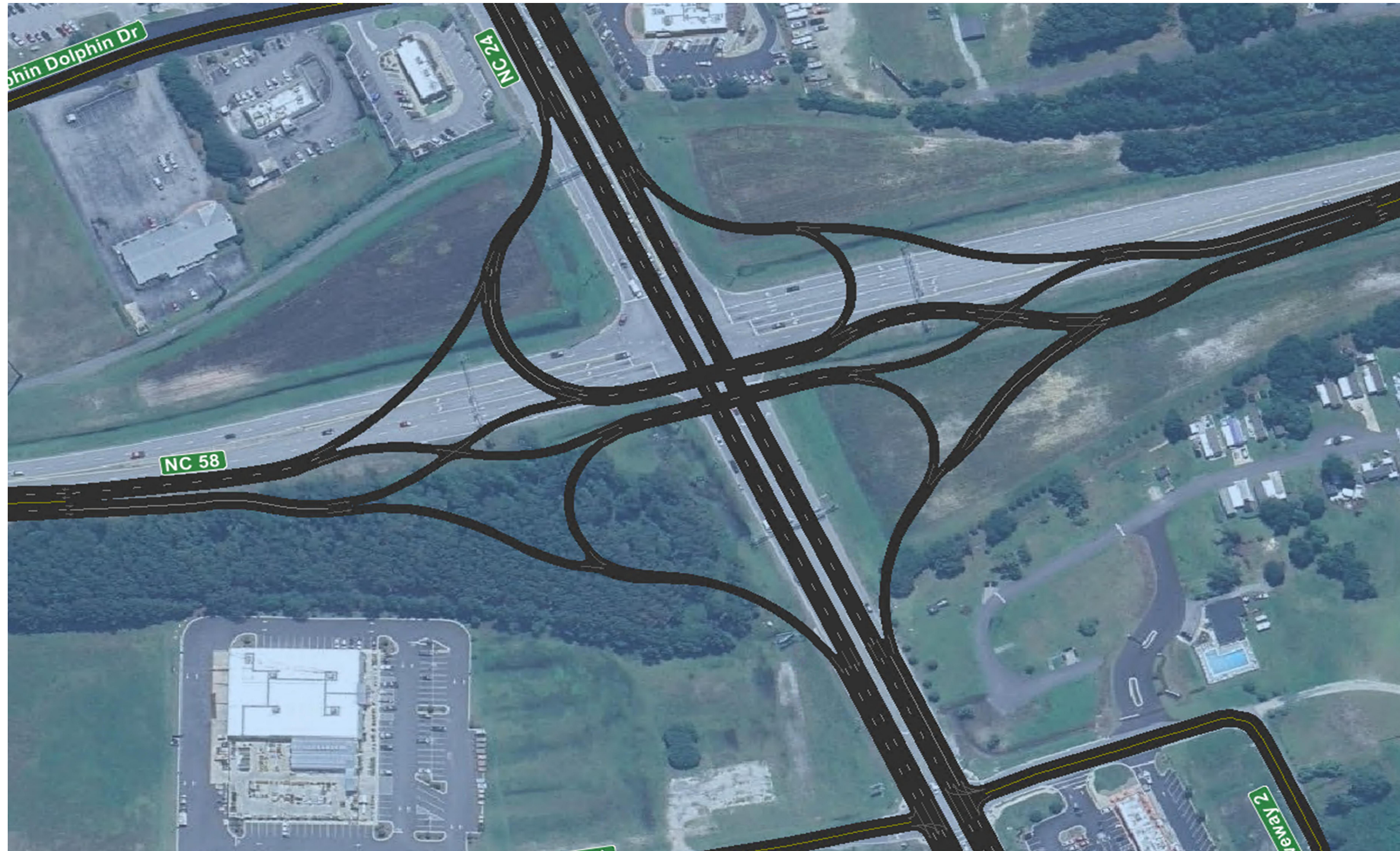
Construct a Diverging Diamond Interchange
